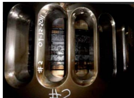
Fig. 16. An example of damage to cylinder rings on an S80ME-C9 engine
