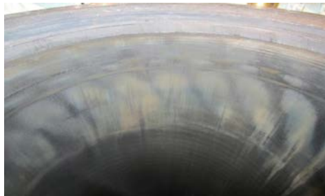
Fig. 15. Example of cold corrosion of an engine cylinder liner
