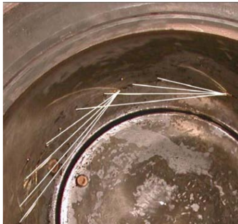
Fig. 6. RPLS cylinder oil injection direction
