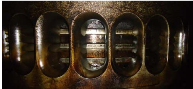
Fig. 12. Example of damage to cylinder rings on an engine
