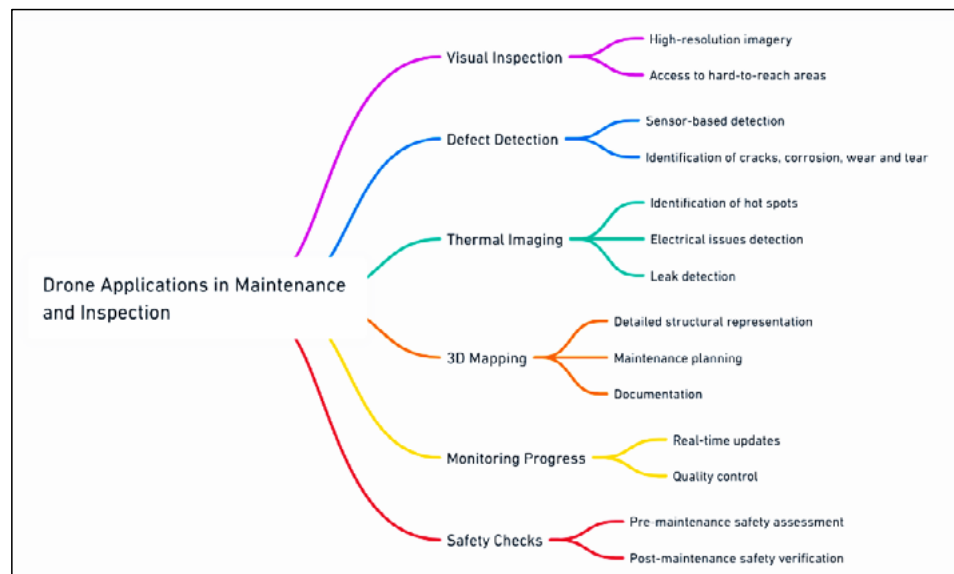
Fig. 2. Mind map of drone applications in maintenance and inspection
